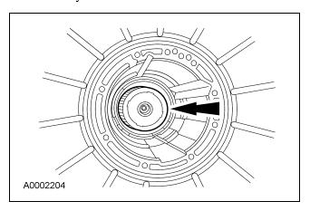
35. Install the No. 6A forward ring gear hub thrust bearing into the forward ring gear and hub.
